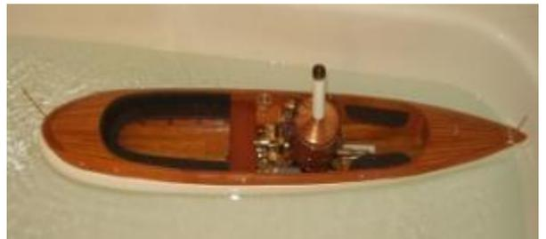
Here the boat is steaming in the bathtub. All the fittings have been attached. The boiler produces about 60 pounds of steam and I think this boat will boogie. However it runs out of gas in about 10 minutes. So it will be a fast but short run.
